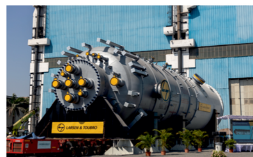
OxO Reactor for BASF Guangdong Integrated Project, China
